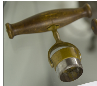
These items, known as "jaggers," would cut out individual hosts from a large sheet of Communion bread.
